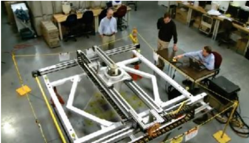
Figure 50: A photograph of the Compton Dry Cask Imaging System.
